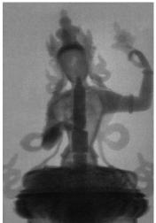
The neutron imaging system at the Czech Technical University in Prague (CTU) revealed an axis mundi (a symbol of the connection between the physical and spiritual worlds) inside a Tibetan Bon statue of Chamma.
