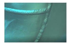
for the safety and operation of reactors. Specialized equipment can monitor structural defects and damage to a reactor's physical infrastructure. These examinations identify cracks, other defects or weaknesses in structures at an early stage and over time in a reactor's concrete and metal parts using radiation resistant underwater cameras and other specialized tools.
