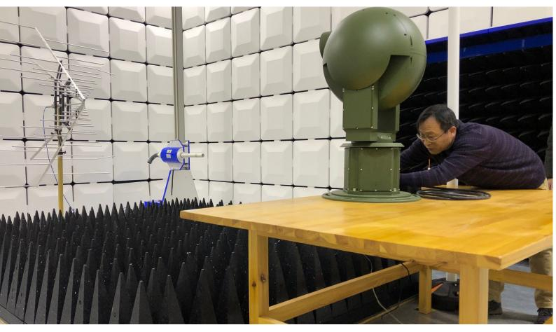
A simulator room in the SNSTC designed to generate and contain strong electromagnetic waves for testing nuclear security equipment.
