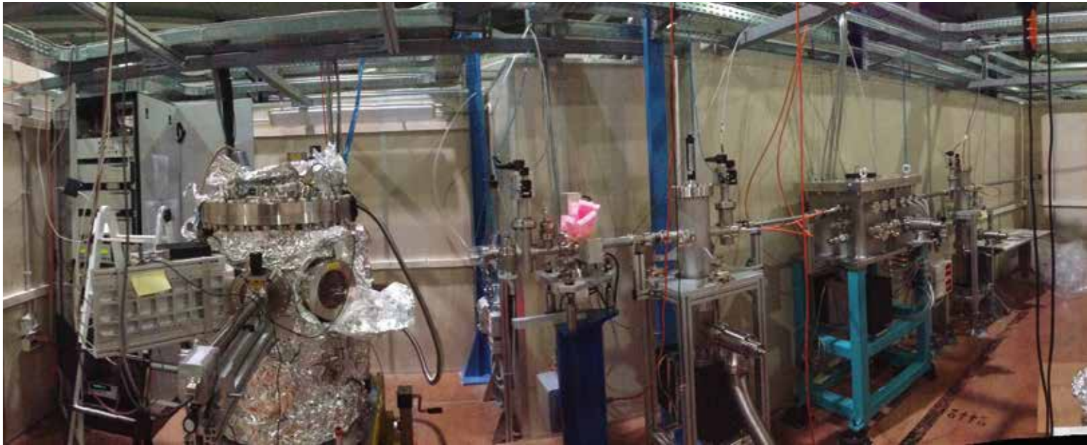
6 A panoramic view of the IAEA beam line at the Elettra Synchrotron Chamber in Trieste, Italy. The synchrotron radiation beam line enters from the right side of the chamber and finally reaches the UHVC, which is the end station seen just left of centre. Synchrotron beam light facilities produce X-rays that are millions of times brighter than medical X-rays. Scientists use these highly focused, intense beams of X-rays to reveal the identity and arrangement of atoms in a wide range of materials, including metals, semiconductors, ceramics, polymers, catalysts, plastics and biological molecules. The IAEA beam line has been working since April 2014. This beam line is especially suited to material science applications. (Photo: IAEA)
