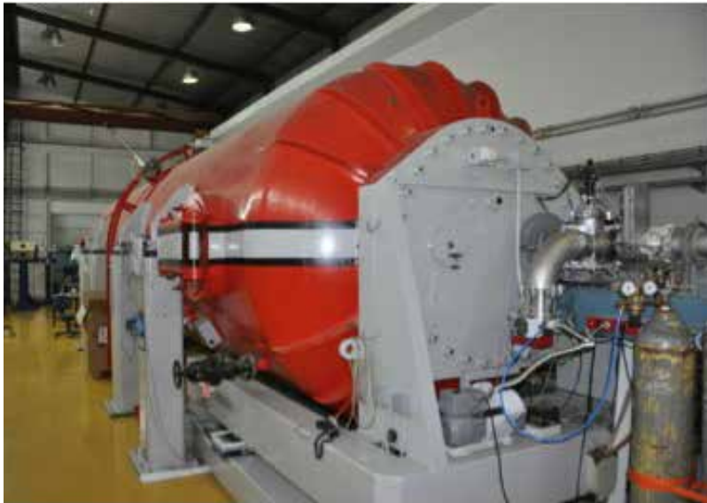
7 Ion beam accelerator at the Ruđer Bošković Institute (RBI) in Zagreb, Croatia. The IAEA NSIL has been operating a beam line at this accelerator since 1996. The accelerator uses a voltage of six million volts to accelerate protons that are used for a wide variety of applications, such as material analysis. (Photo: RBI, Zagreb)
