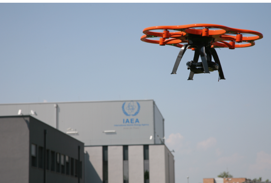
Unmanned aerial vehicle designed by NSIL for remote environmental radiation monitoring. (Photo: Steve Thachet, IAEA)
