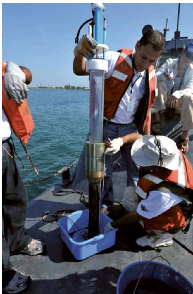
8 Scientists first check that the quantity and quality of the samples are adequate for laboratory testing. Should the sediments contain impurities, they are returned and the process begins anew. Once the sediment samples are determined to be of good quality, the process of removing the corer from the plastic cylinder begins.
