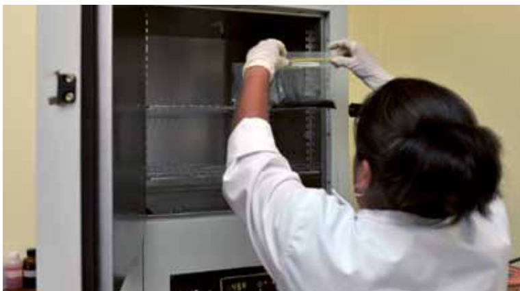
13 Other members of the team then label and tag the sediment sample according to color, texture, smell, etc. Later, samples are dried at controlled temperature in an oven before being shipped to participating laboratories that will analyze them.
