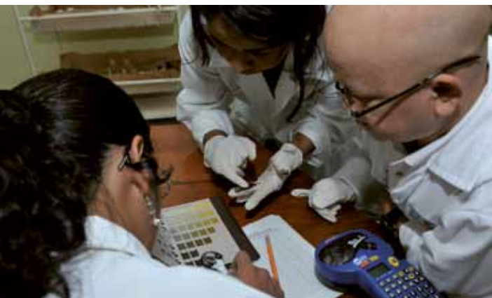
13 Other members of the team then label and tag the sediment sample according to color, texture, smell, etc. Later, samples are dried at controlled temperature in an oven before being shipped to participating laboratories that will analyze them.
