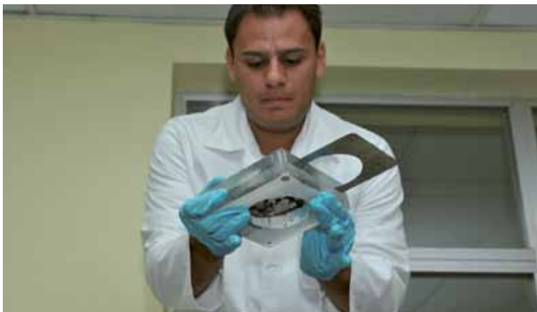
12 Preparing the samples for analysis is a complex process that requires varied tasks. Here, Dr. Dennys Canales-Cruz, Honduran project team leader, carefully removes a slice of the sediment sample from the vertical core.
