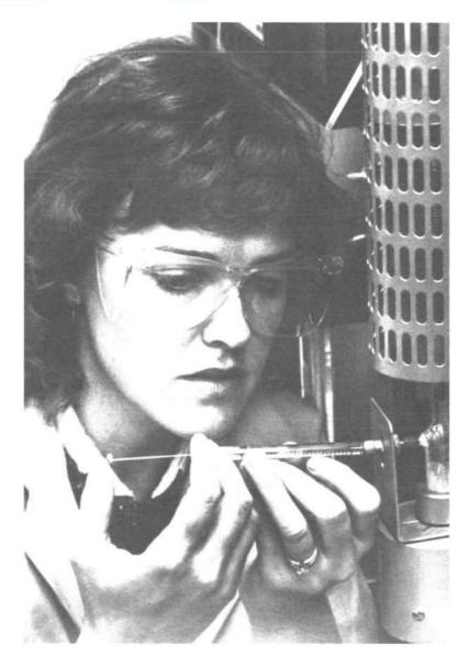
realizing future opportunities. It is for the sake of improving safety, reliability, and economics that the challenge to move towards performance– based QA programmes is encouraged. Water tests by chemistry technicians at nuclear plants help prevent corrosion of components. (Credit INPO)
