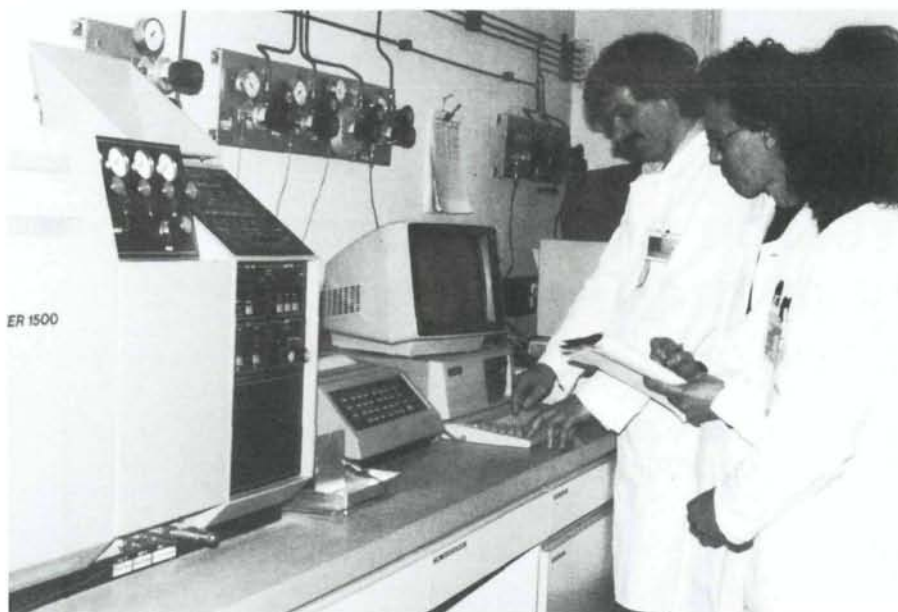
Advanced instrumentation available at the Soil Science Unit — such as an automatic nitrogen analyser coupled to a stable isotope ratio analyser — permits an increased sample throughput for routine analytical services in support of the field projects of the Joint FAO/IAEA programme.
