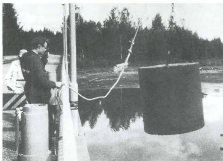
In Finland, extensive research has been conducted for nuclear waste disposal. As part of site investigation studies, a geophysical airborne survey was done. Computer codes are used for studies of groundwater movement. Additionally, full-scale concrete waste containers were submerged in a river for 5 years to test their properties. (Credit: YJT, Finland)
