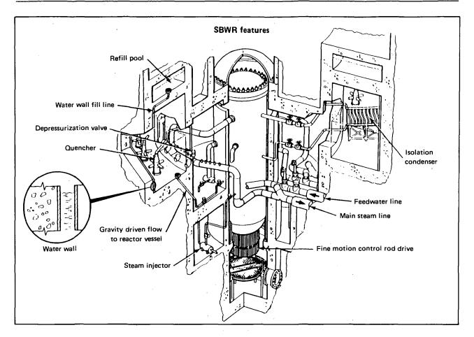
The SBWR reactor is designed for operation at full power without recirculation pumps. Elimination of recirculation pumps and piping permits a simpler reactor vessel design, reduces vulnerability to LOCA events, and reduces maintenance requirements. The larger reactor vessel needed for natural circulation provides the additional benefit of greater inventory of water over the core at the initiation of any upset conditions.
