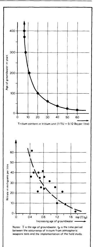
These figures show the correlation between nitrate and tritium concentration observed in an unconfined Permian aquifer in the German Democratic Republic. The correlation indicates that the nitrate has been transported into the groundwater by the infiltration of rain water.
