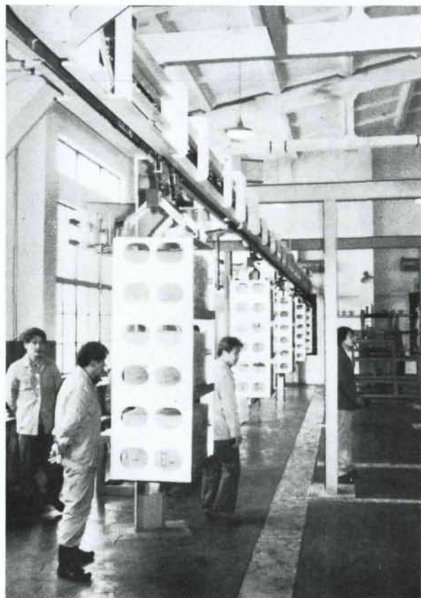
Racks of boxed apples move automatically to the irradiation chamber at the Shanghai facility. (Credit: Wedekind)
