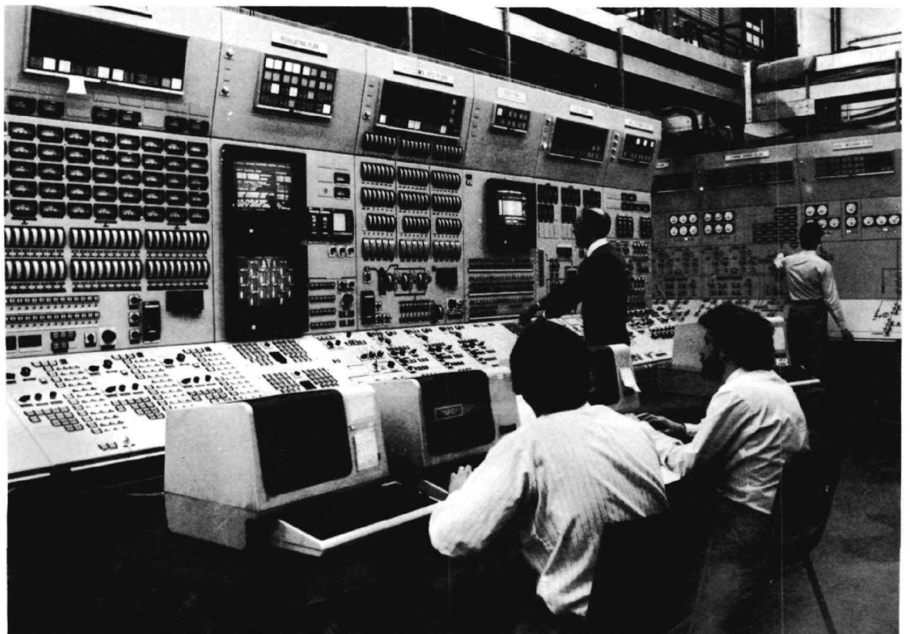
Plant-specific simulators are replicas of a particular control room. Shown are the systems for the Susquehanna nuclear plant in the USA (top) and for the Ontario Hydro Bruce "B" CANDU power plant in Canada. (Credit top photo: Link SSD; bottom: CAE Electronics Ltd.)
