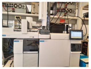
Gas chromatography/mass spectrometry (GC/MS) which was provided by the IAEA to the Institute of Marine Affairs and is being utilized for the analysis of petroleum hydrocarbons, including polycyclic aromatic hydrocarbons, as well as fingerprinting oil spills. This has been instrumental in assisting the country in conducting analysis during the recent oil spill which occurred in February 2024. (Photo: I. Tolosa/IAEA)
