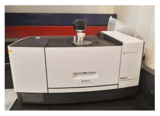
Infra-red spectrometer for microplastic monitoring, provided by the IAEA to the Institute of Marine Affairs, as part of the support to strengthen the institution's analytical capabilities in relation to the marine environment. (Photo: I. Tolosa/IAEA)
