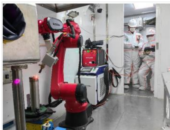
Fig.2 Remote control welding
