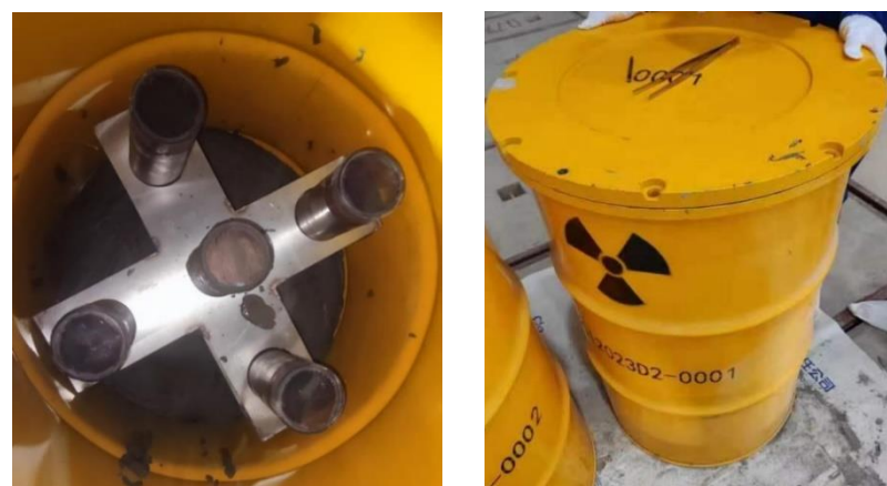
Fig.3 DSRS packages (200L metal drum with brackets)
