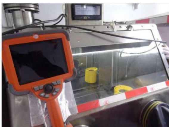
Fig. 1 Glove box used in conditioning DSRS
