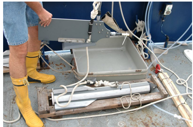
Figure 3. Surface pump sipper/tow fish system (GEOTRACES, 2017)
