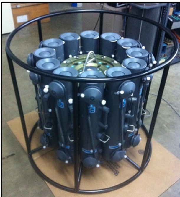
Figure 1. Individual GO FLO seawater sampler and rosette system with multiple samplers
