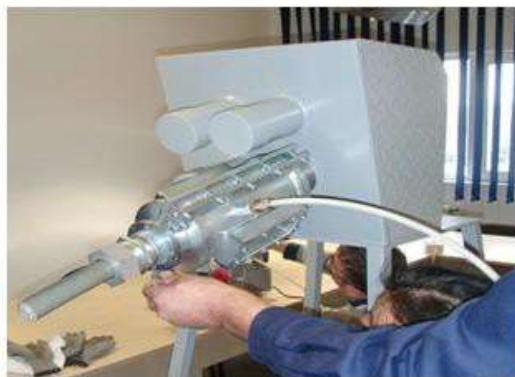
Figure 3 - Mock-up with vacuum box installed
