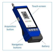
Figure 44: Prototype of a unified seal reader under MSSP Task EC E 2008 (Identification, Development, Testing and Vulnerability Assessment of Sealing Technologies for International SG).
