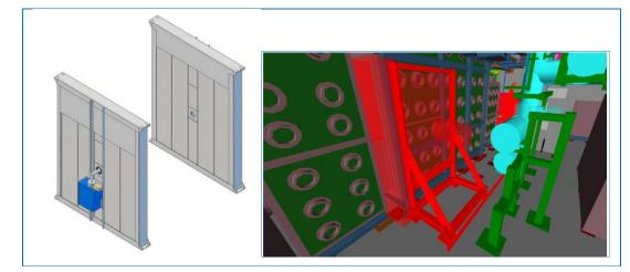
Figure 62: Advanced Material Accountancy Glove Box NDA system.
