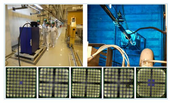
Figure 73: Testing of the Unattended Gamma Emission Tomography (UGET) at the interim Spent Fuel Storage at the Olkiluoto Nuclear Power Plant (Finland).
