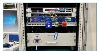
Figure 76: A prototype of an active security system installed in the mediumsize cabinet.
