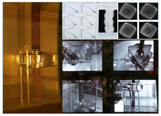
Figure 74: The Passive Gamma Emission Tomography (PGET) system's performance evaluation on the Boiling Water Reactor (BWR) spent fuel in a hot cell at Zwilag (Switzerland).
