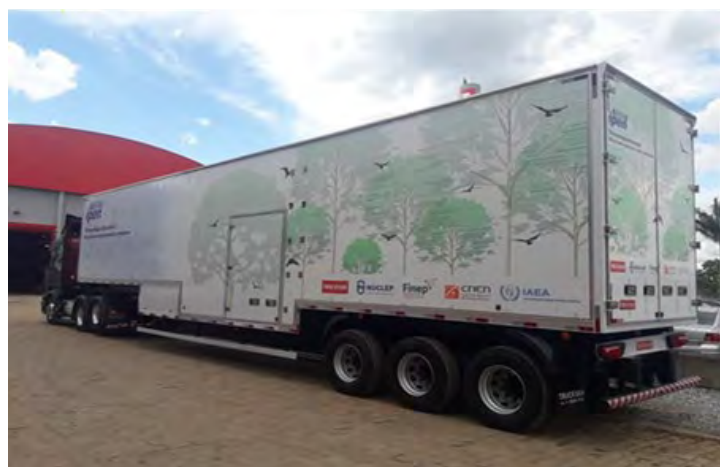
FIG. 1 - Mobile electron beam irradiation unit for the treatment of industrial effluents in Brazil.
