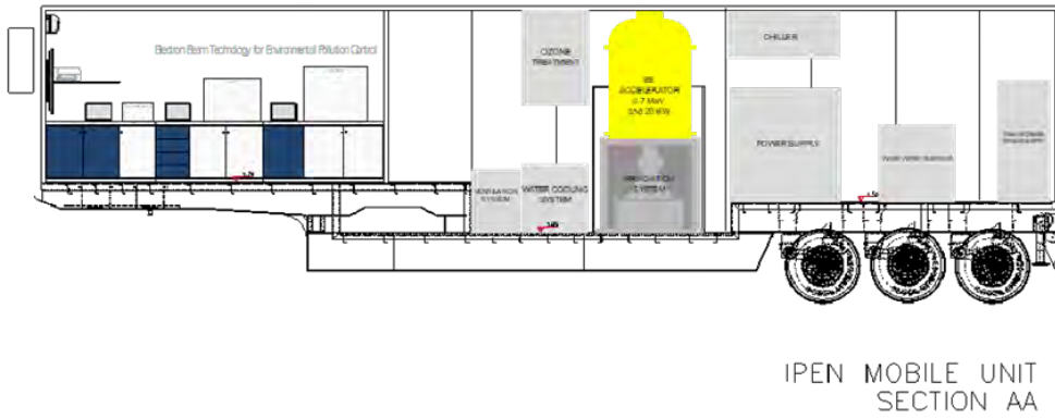
FIG. 2 - Architectural drawings of the IPEN-CNEN mobile unit (a) Plan and (b) section AA (15m length, 2.6m width and 4.4m height).
