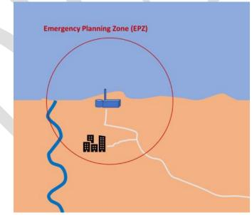
FIG. 2. Example of an unsuitable site — a physical barrier (river) preventing construction of an alternative evacuation route in another direction – site unsuitable if a bridge is not constructed or alternative evacuation route.
