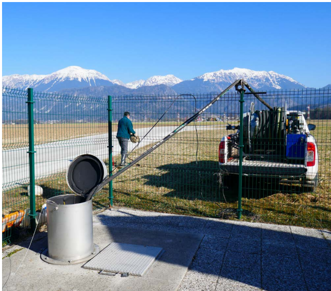
Pumping a groundwater well close to Radovljica, between the Julian Alps and Karavanke Mountains. (Photo: Nina Rman)
