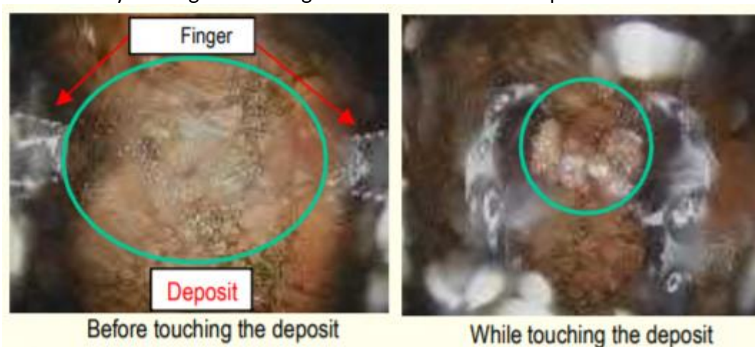
Image: Before and while touching the deposit at the investigation of Unit 2
