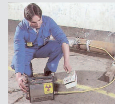
A radiographer checking that the radioactive source is safe.
