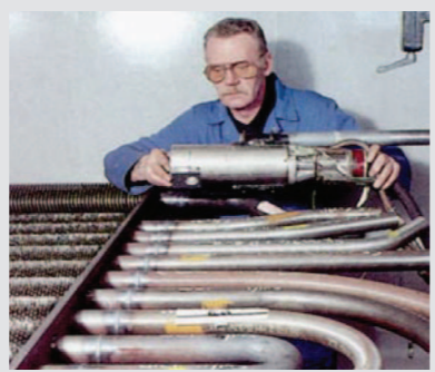
A radiographer positioning the object and X ray machine.
