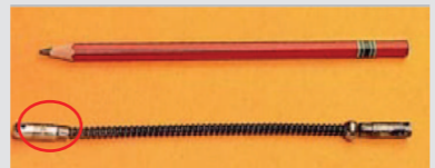
Radiography sources are typically incorporated into 'pigtails'. The pigtail may be about the same size as a pencil but the actual source (circled, above) is physically smaller.
