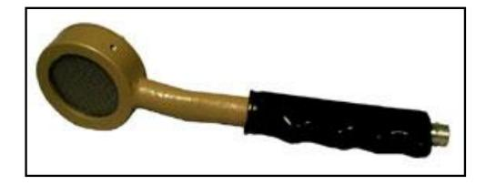
Pancake halogen quenched GM tube. Window =  $12 \text{ cm}^2$ Efficiency = 15 % for  $^{239}$ Pu
