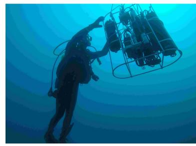
IAEA researchers measure parameters such as sea temperature and salinity to increase their understanding of the global carbon cycle and factors which can impact it. (Photo: R. Cassi/IAEA)
