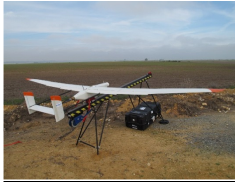
Figure 4: Fixed-wing UAS with MTOW < 25kg.
