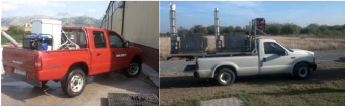
Figure 11. Illustration of pick-ups used to carry automated ground release systems for Ceratitidis capitata in Croatia and Mexico.
