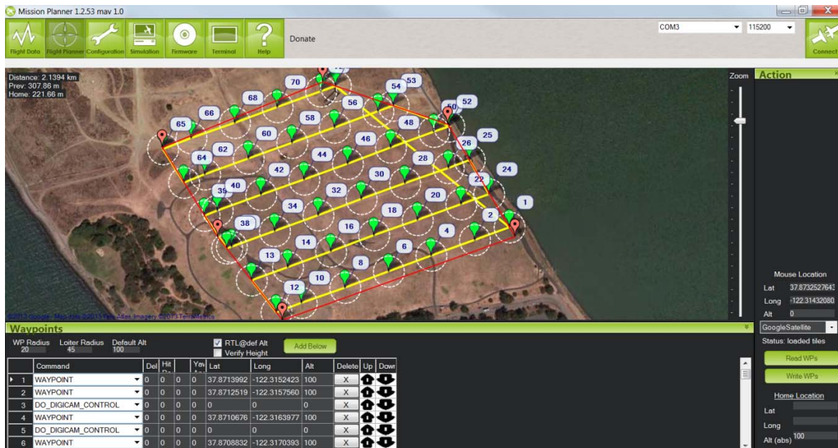
Figure 9. Example graphic showing a set of waypoints over a path, from the 3.2.3. GIS dose release method for aerial release.
