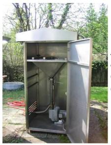
Aerosol Sampler 88 Nm<sup>3</sup>/h Glass microfiber filter GF/A
