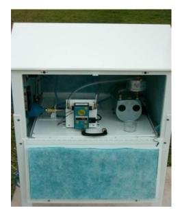
Iodine Sampler 4.5 Nm<sup>3</sup>/h Carbon Cartridge, Glass fiber filter
