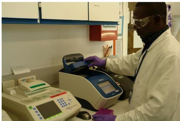
FIG. 8. PCR machine with heated lid to set up the PCR reactions.
