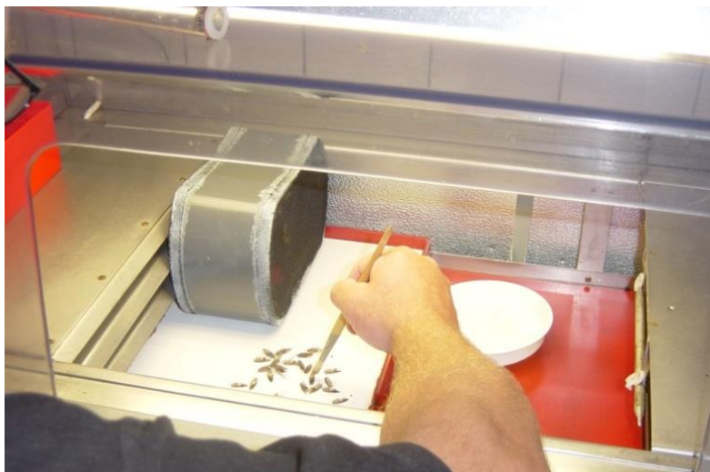
Figure 8. Chillers showing an emergence cage and adults immobilized by the cold during sex separation
