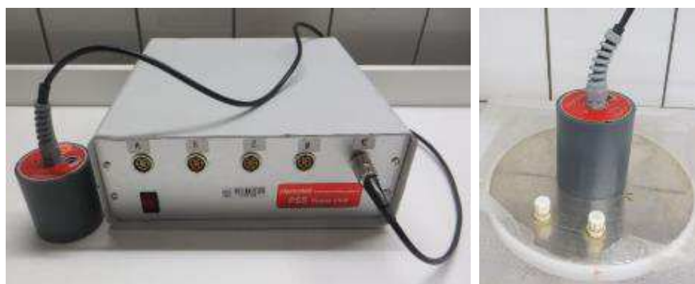
Figure 12. The hemotek membrane feeding system (discovery workshops, lancashire, united kingdom). The hemotek power unit with a feeder (left) and the modified aluminium plate with the much larger surface area attached to a feeder (right).
