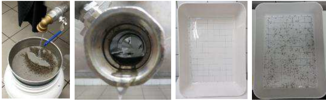
Figure 14. Draining waste from the cages. From left to right: waste water container with a sieve on top to collect debris; view inside the spout where mosquitoes may cluster and block the flow; an empty tray with grid markings and a tray filled with dead adults for counting.
