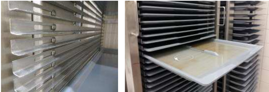
Figure 18. Mass-rearing rack. The shelves that facilitate a sliding and tilting mechanism for the large plastic trays (left); the large plastic trays stacked in the steel rack (right) complete with water, larvae and diet slurry.
