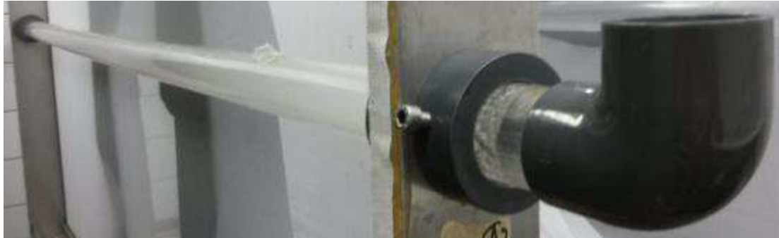
Figure 6. The internal sugar feeding device. The device spans the entire width of the mass-rearing cage. The sugar solution is poured through the open elbow plumbing fixture into the tube and can last up to 20 days.
