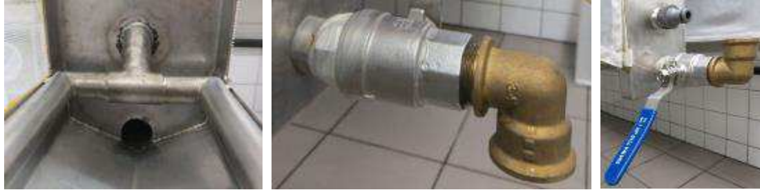
Figure 4. The drainage system. View of the water pipe system and the water outlet from inside the cage (left); the stopcock with the elbow plumbing fixture down (open position) to drain water (middle); the stopcock with the elbow plumbing fixture up (closed position) to load the cage with pupae (right).
