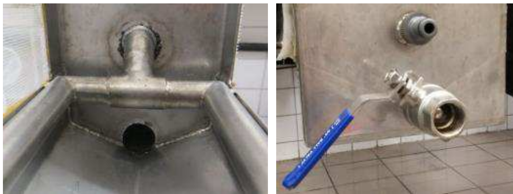
Figure 15. Internal irrigation system. View of the spout outlet from inside the cage (left) and the hose pipe and stopcock from outside the cage (right).
