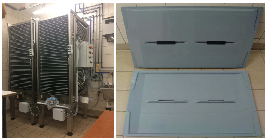
Figure 9. A large rearing tray (right) and rack unit (left).
