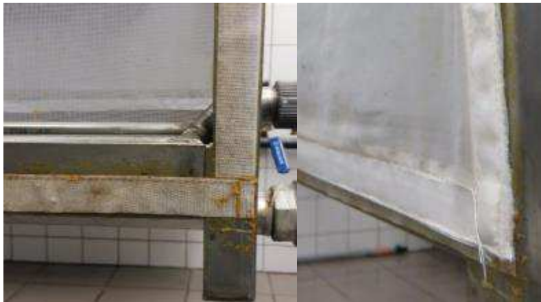
Figure 7. The detachable netting system using velcro® tape. A corner of an open cage aligned with velcro® taping (left). The net is taped onto the cage by pressing it
