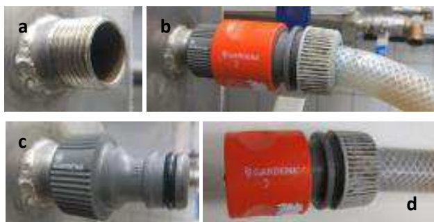
Figure 3. Components of the hose pipe system. (a) the cage's open valve as it is when it's delivered; (b) the whole hose pipe system attached to the large cage; (c) the grey (+/male) connector fixed to the open valve; (d) the water
