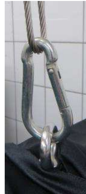
Figure 5. A carabineer attached to the top of the cage. The cage is suspended on a cable hanging from the ceiling. The black cloth shroud is draped over the cage so that the carabineers emerge from the holes and the black cloth covers the cage.
