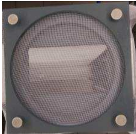
Figure 8. The blood feeding port. A membrane filled with blood can be placed on top of this net-covered panel to provide mosquitoes with blood.
