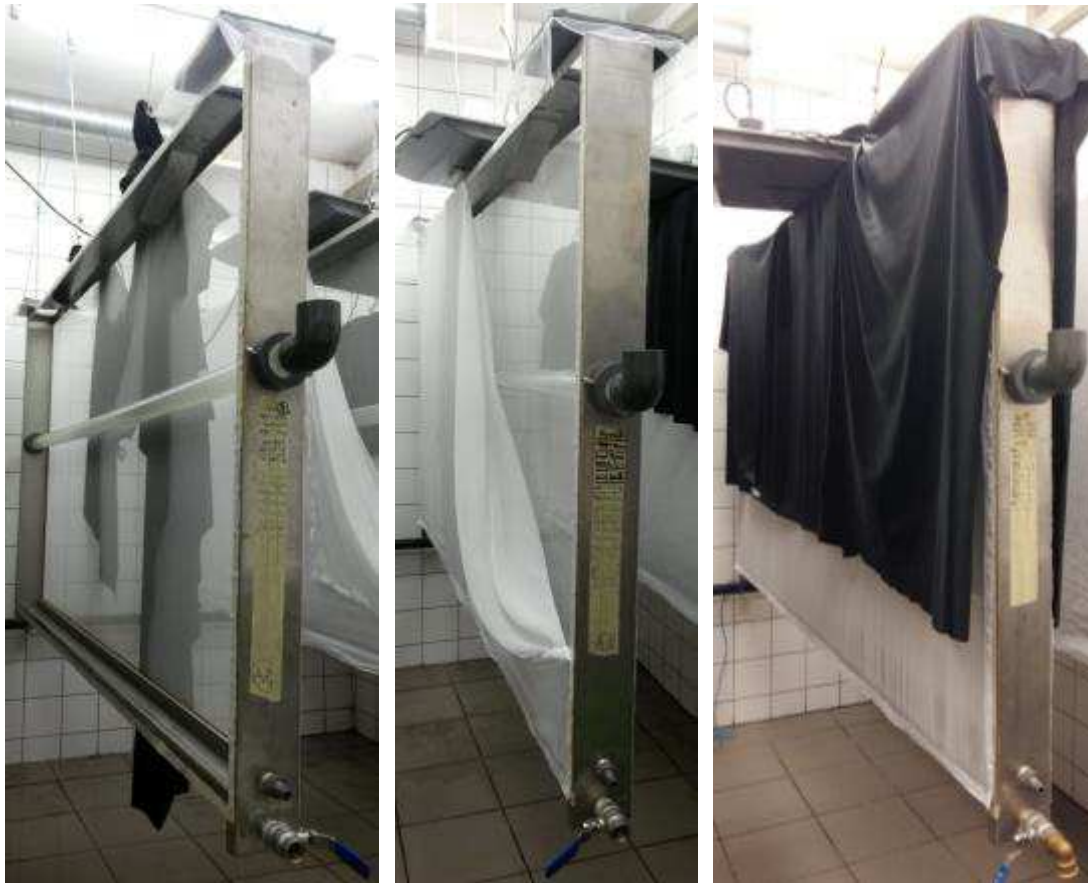
Figure 10. A large cage: without the net prior to adding pupae (left), with the net partially attached after loading the pupae (middle) and fully assembled with the net and black lining (right).
