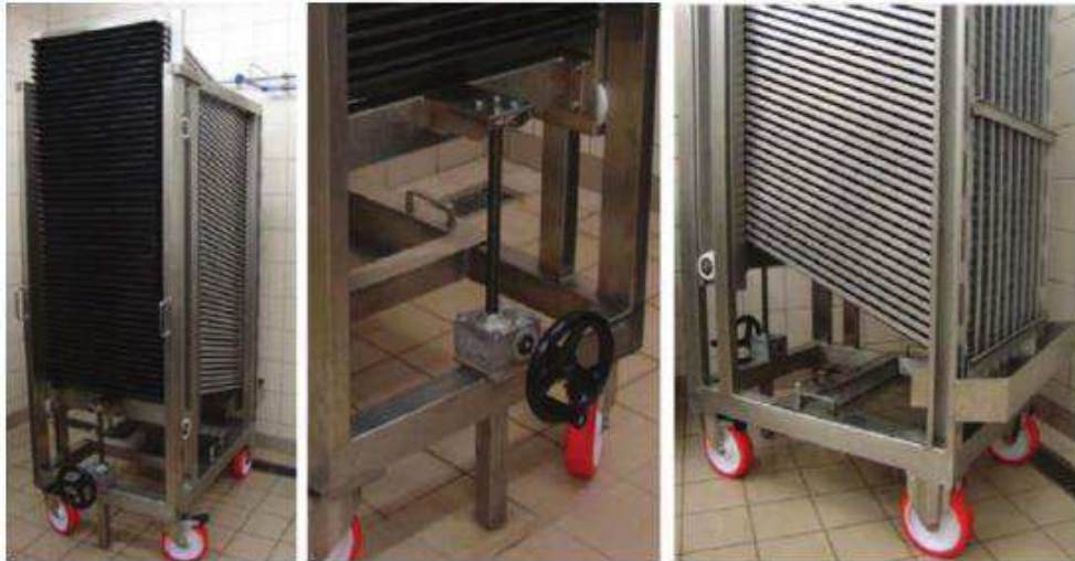
FIGURE 21. The stainless steel rack system (left), the screw jack at the base of the rack (middle) and the trays in a tilted position (right).
