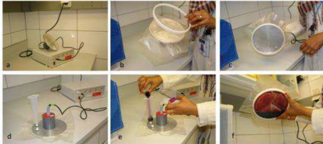
Figure 13. Setting up the hemotek membrane feeding system.
