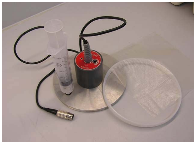
Figure 43. Blood feeder plate connected to the Hemotek heater and the syringe used for blood replenishment. On the right is shown the membrane employed and the plastic ring to fasten it to the plate.
