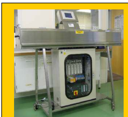
Figure 1. UV irradiator for tsetse blood
