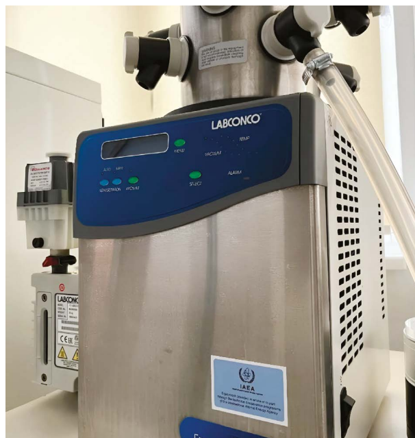
Equipment provided by the IAEA to perform freeze drying — a dehydration process typically used to preserve perishable materials or make them more convenient for transport (Photo: Institute of Veterinary Medicine in Serbia)
