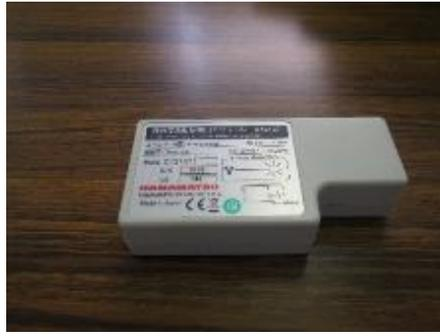
Figure 17. High-dose CsI detector (Hamamatsu Photonics C12137)
