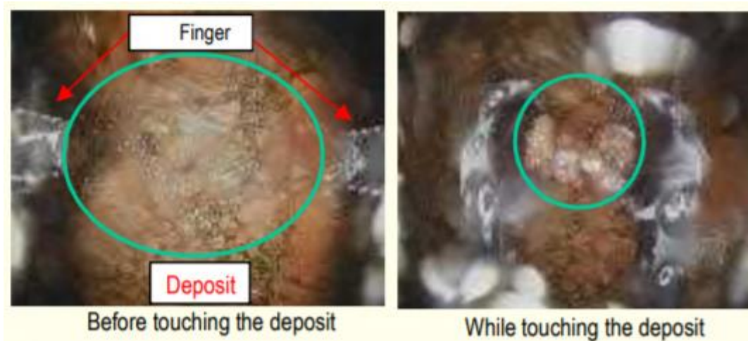
Image: Before and while touching the deposit at the investigation of Unit 2
