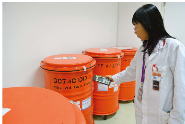
An IAEA Radiation Monitoring Technician from Singapore measures the photon ambient dose equivalent rate on the outside of transport containers ready for shipment. (Photo: D. Calma/IAEA)
