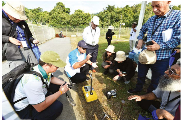
A demonstration of a nuclear density gauge. (Photo: Malaysia Nuclear Agency)
