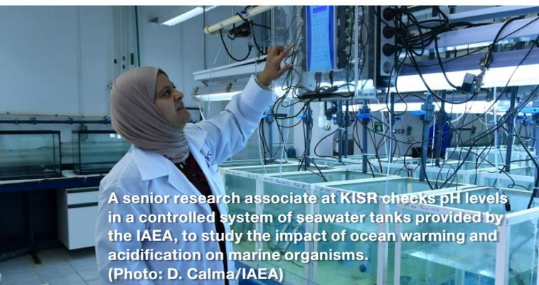
A senior research associate at KISR checks pH levels in a controlled system of seawater tanks provided by the IAEA, to study the impact of ocean warming and acidification on marine organisms. (Photo: D. Calma/IAEA)
