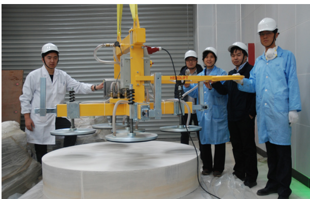
Scientists at Beijing's Research Institute of Uranium Geology, test a bentonite block which acts as a buffer for high-level radioactive waste. The IAEA provided technical assistance and staff training in geological, geohydrological and mechanical studies for waste disposal. (Photo: G Cheng/BRIUG)
