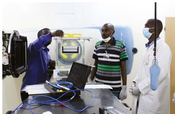
Calibration of a radiotherapy machine at the National Cancer Institute in Sudan. (Photo: SAEC)
