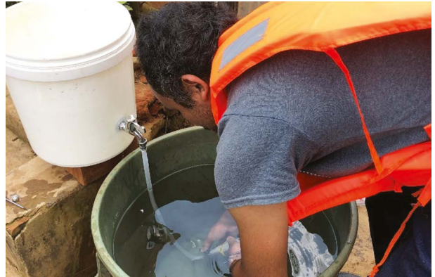
Water sampling for CFC (Chlorofluorocarbon)/SF6 (Sulfur Hexafluoride) analysis in Ambohimambola-Madagascar. (Photo: INSTN-Madagascar)
