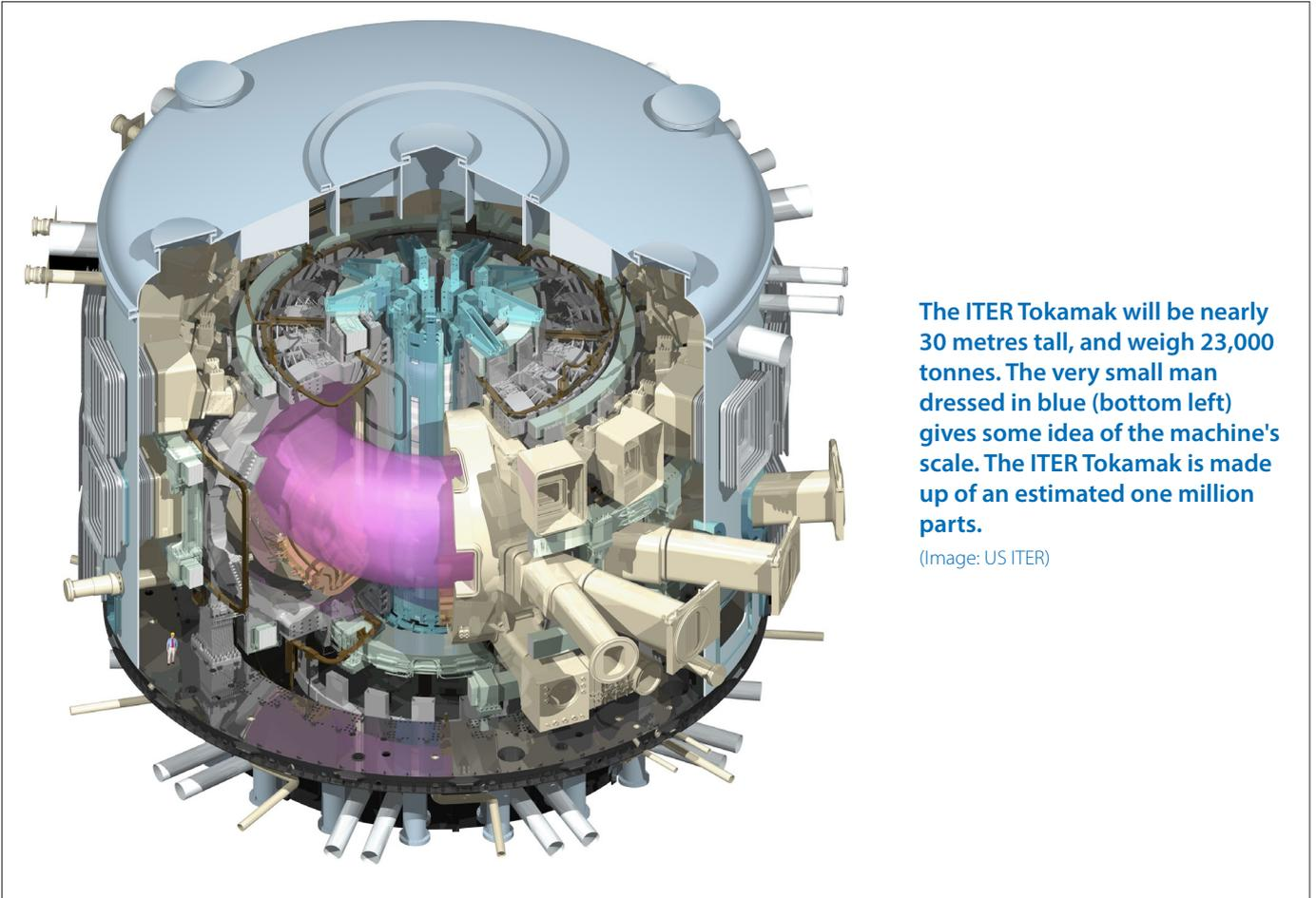
The ITER Tokamak will be nearly 30 metres tall, and weigh 23,000 tonnes. The very small man dressed in blue (bottom left) gives some idea of the machine's scale. The ITER Tokamak is made up of an estimated one million parts.
