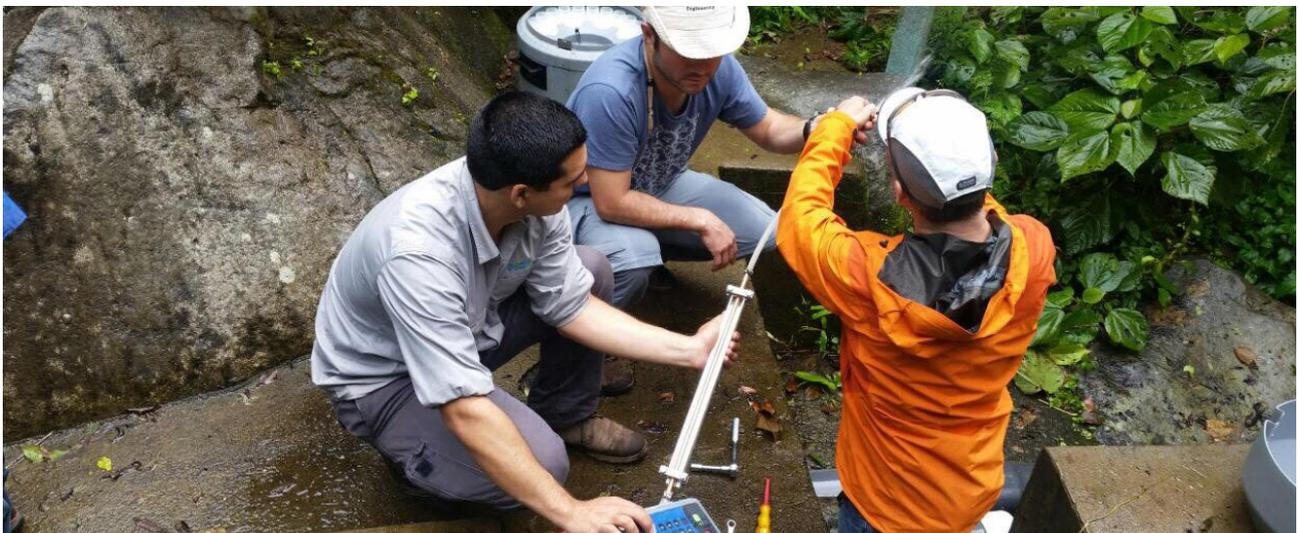
Sample preparation for noble gases analysis of spring water. (Photo: L. Castro/ESPH).
