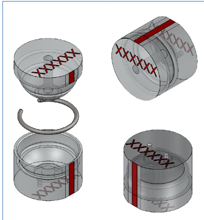
*Figure 1. Latest design of the Glass Seal (GLAS) with a new self-aligning round bottom avoiding breaking on closure*
