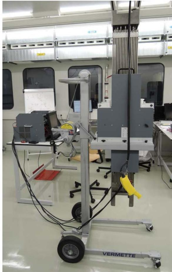
*Figure 4&5. Fact Neutron Coincidence collar is undergoing performance evaluation on the fuel containing burnable poison rods*
