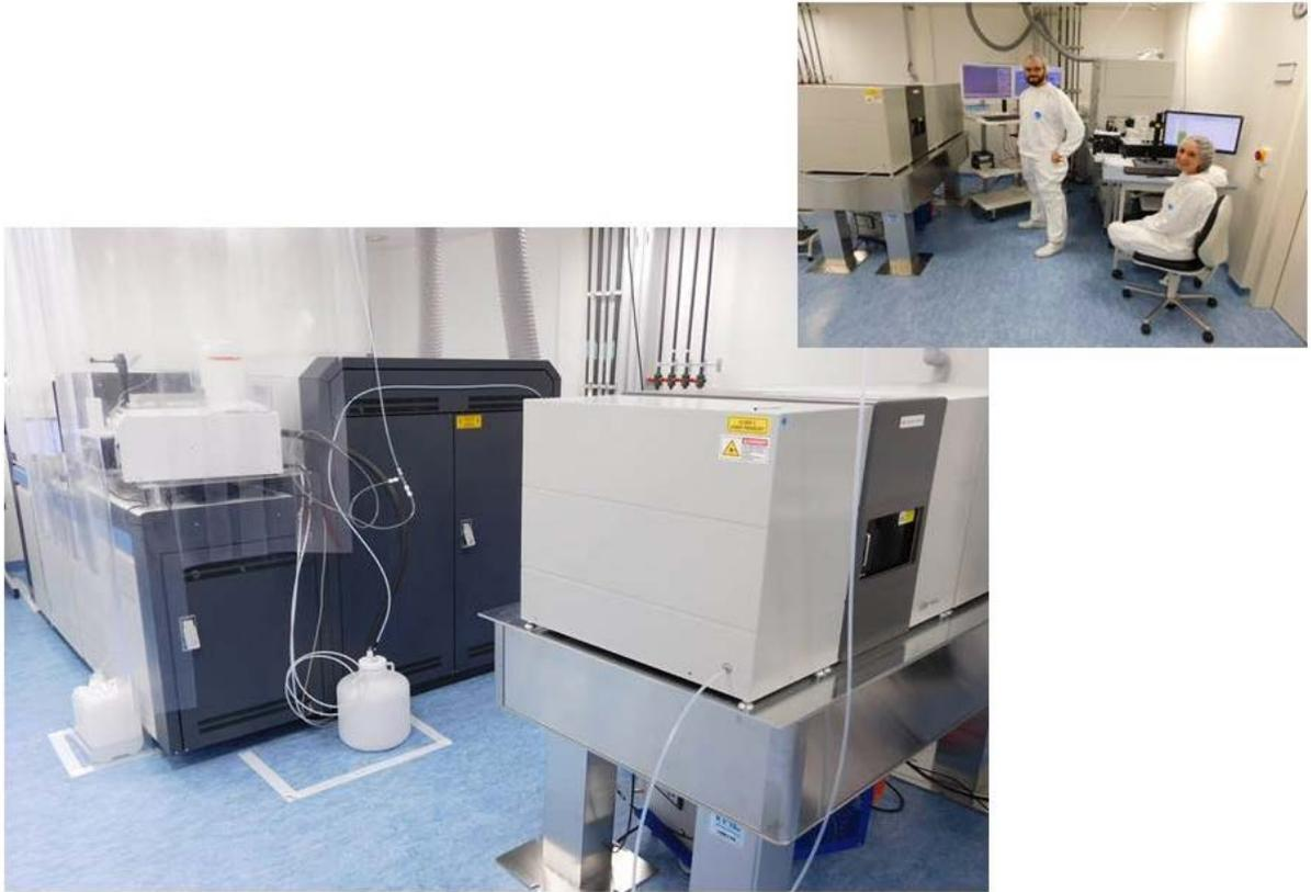
*Figure 1: Femtosecond Laser Ablation System coupled to MC-ICP-MS for the analysis of particles and other solid matrices*
