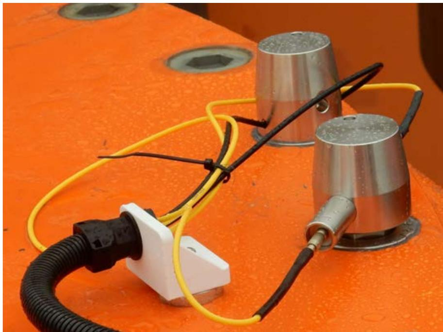
*Figure 2. The Ultrasonic Optical Sealing Bolt (UOSB) installed at a spent fuel storage facility saving significant inspector and facility resources*
