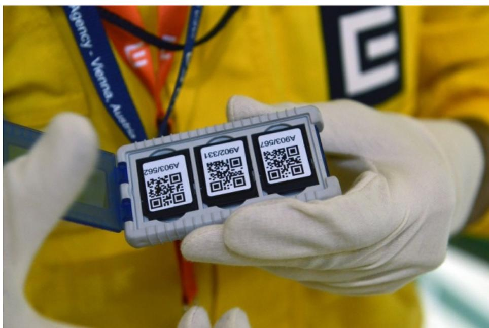
*Figure 2: Radiation-tolerant SD cards deployed with next generation surveillance systems (NGSS) in elevated radiation environments*
