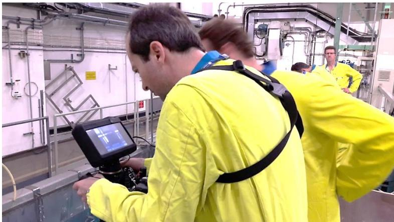
Figure 4. Cerenkov Viewing Device (XCVD) field test at Ringhals
