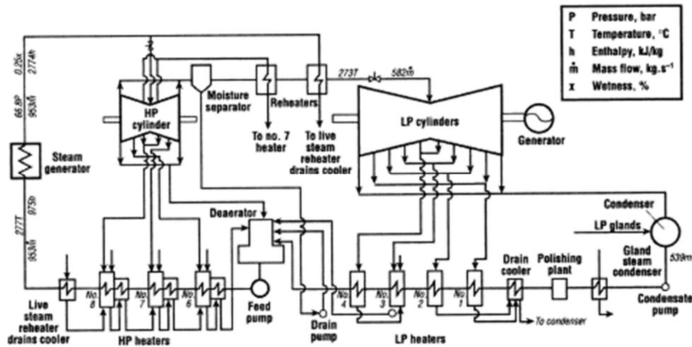
Figure 3 Schematic diagram of a large nuclear power unit secondary cycle
