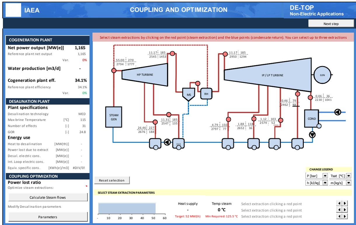
Figure 10 DE-TOP Coupling configuration screen. Red points in the flow sheet diagram are possible steam extraction points. Blue points represent possible location of condensate returns
