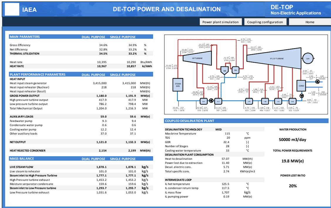
Figure 16 DE-TOP Final report for the combined power and MED thermal desalination plant.
