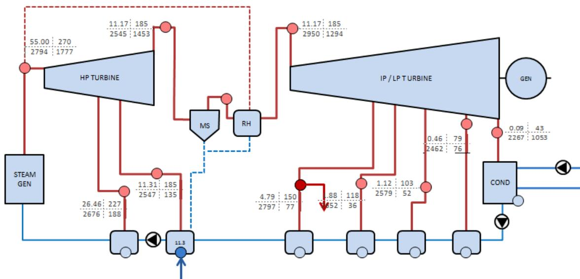
Figure 12 Flow sheet diagram after selection of the extraction and condensate return.
