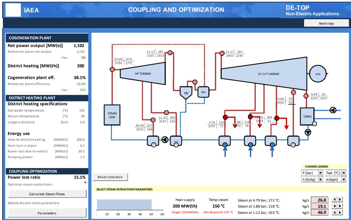
Figure 15 Coupling configuration for district heating application, example for multiple extraction points.
