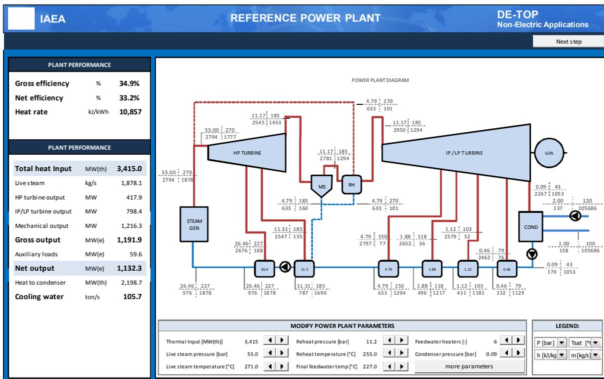
Figure 7 Results of the simulation for the reference power plant.
