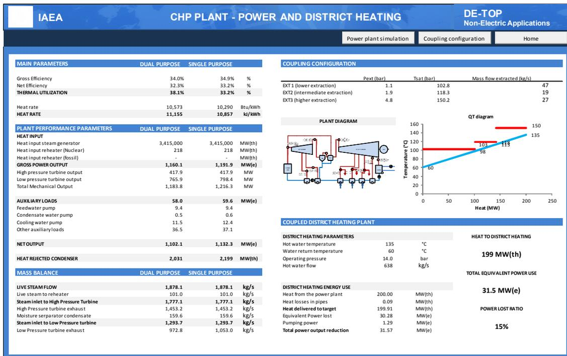
Figure 17 DE-TOP Final report for the combined heat and power plant with district heating application.
