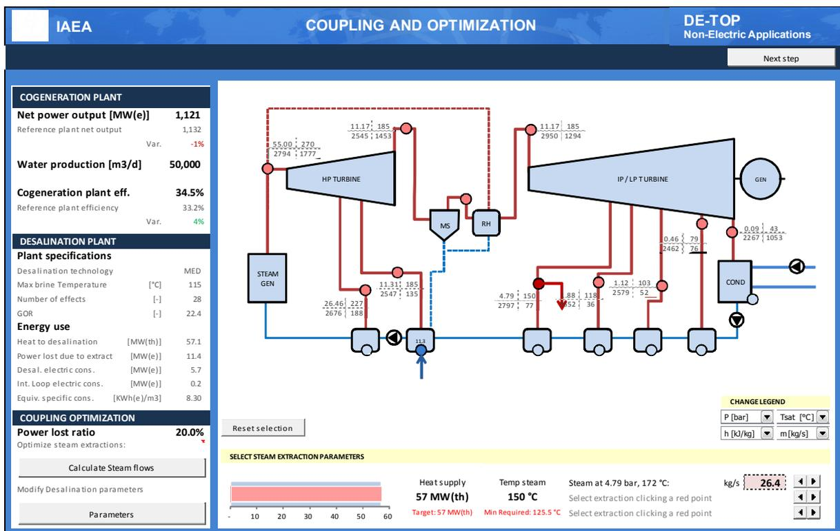
Figure 14 Selected coupling flow sheet. Cogeneration plant parameters are shown on the left column. The Power lost ratio acts as an indicator and gives an idea of how optimized is the user selected lay-out.
