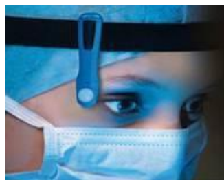
FIG. 2. The EYE-D dosimeter holder as close to the eye as possible, attached to a headband
