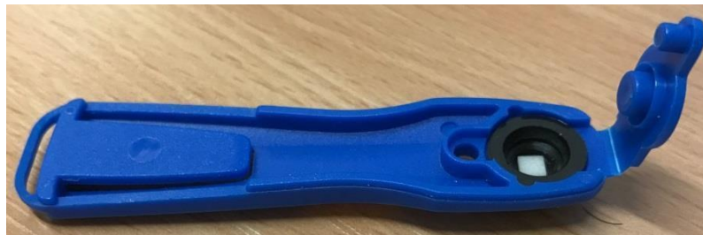
FIG. 1. The EYE-D holder with a TLD inside the capsule
