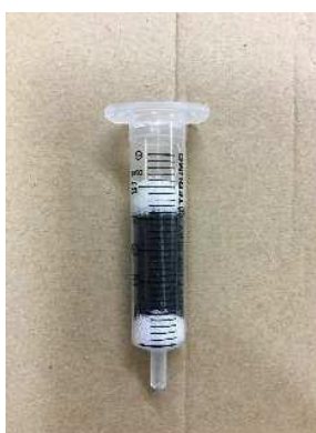
Fig. 1. In-house charcoal column
