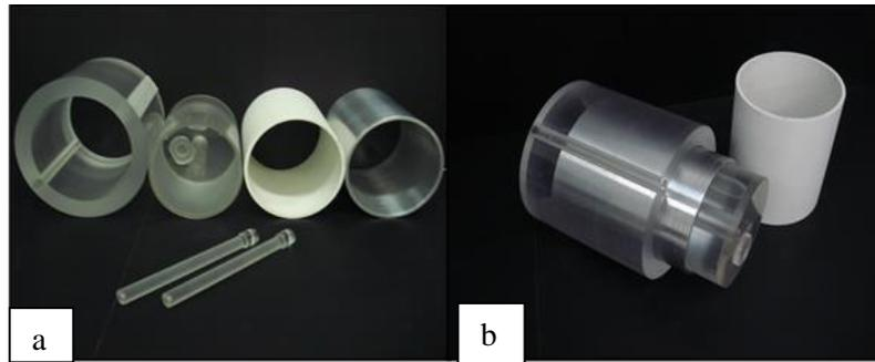
FIG. 2. Pediatric head phantom: a) separated pieces and b) mounted with the aluminum cylinder; the PVC cylinder is outside
