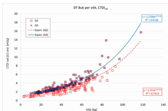
Figure 2. CTDIvol (mGy) as a function of patient weight for CT abdomen examinations. Q2 (red quadrants) and Q3 (blue crosses). Total number of examinations are 304 from four hospitals. All CTDIvol values are for 32 cm PMMA phantom. [3]
