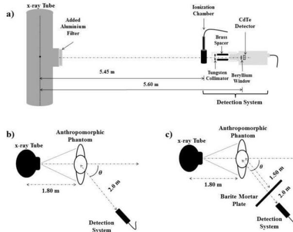
FIG 1 – Experimental setup used to measure (a) primary x-ray spectra, (b) secondary x-ray spectra and (c) transmitted x-ray spectra through a barite mortar plate. The representations of the setup components for each case are not in the real scale [10].
