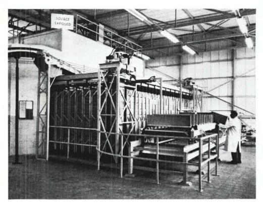
A commercial radiation sterilization plant for medical products at the Gillette Research and Development Laboratory, Reading, Berks., UK. Photo: Gillette
