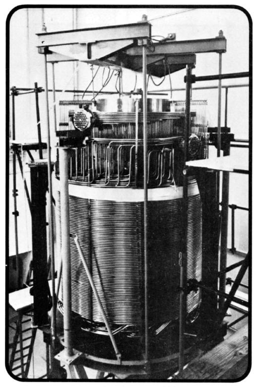
Fig. 1. Steam generator of N.S. Otto Hahn. Credit: Interatom
