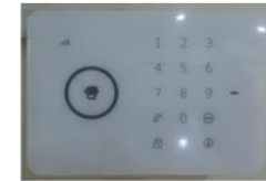
Alarm Control Panel
