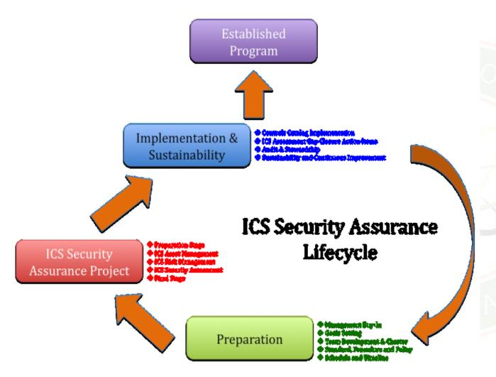
• The CSP follows the ICS cyber security life cycle programme as show in figure 2 to put the required technical, process and management controls used to protect the identified systems against cyber-attacks [6,8]. The CSP requires regulatory approval before it can be executed in the implementation phase and also if future plan modifications are required
